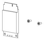
2、Fit LTE module into the corresponding socket base with its "U" slot end facing towards the base and the other end with main terminal facing in opposite direction.
