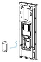
3. Lock the LTE module onto the back cover using two M2 x 4 Machine screws, and press the Coaxial cable terminal into the socket marked with "MAIN" on the module.
